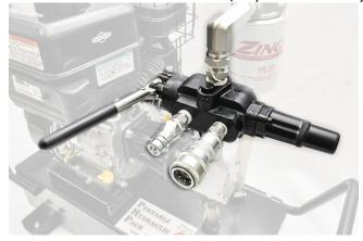
couplers. Be sure your implement is compatible with these couplers. If they are not, we recommend replacing the couplers on the implement rather than using an adaptor, which causes pressure loss.
